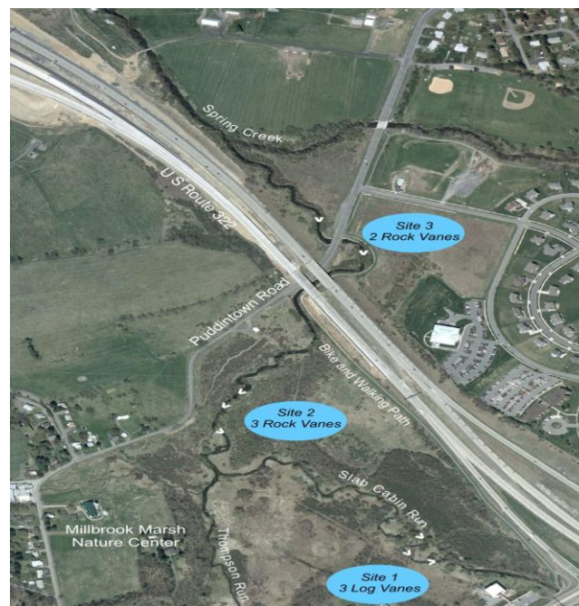
Figure 11. Map of Millbrook Marsh showing locations of cross vanes and monitoring sites. Courtesy of T. Rightnour.
